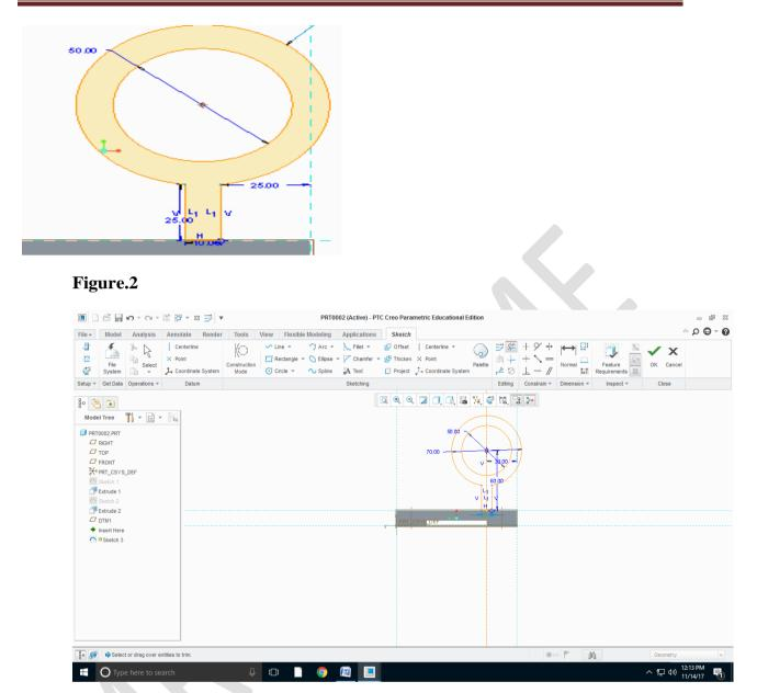
Step9: Extrude the sketch by using Symmetry option and specify the width and direction of extrusion and Click on ok
