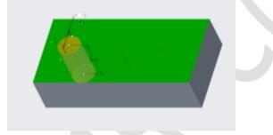
Step8: Create the datum plane at the distance 40 mm from one end of the surface along the length of the sketch and with this as a reference plane draw the required shape of the object and Click on ok
