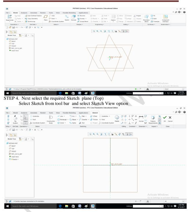
Step 5: Sketch a 2Dprofile of the model as shown in Figure.1 as per the dimensions and Click on ok
