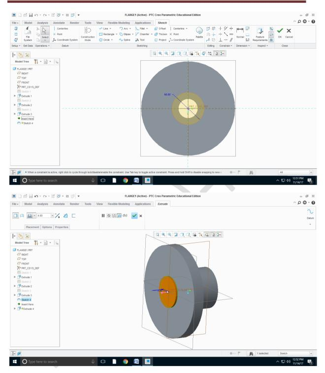
Step9:select the required surface to remove the material in the hub and then draw the shaft in 2d sketch plane and extrude it by giving the required dimensions
