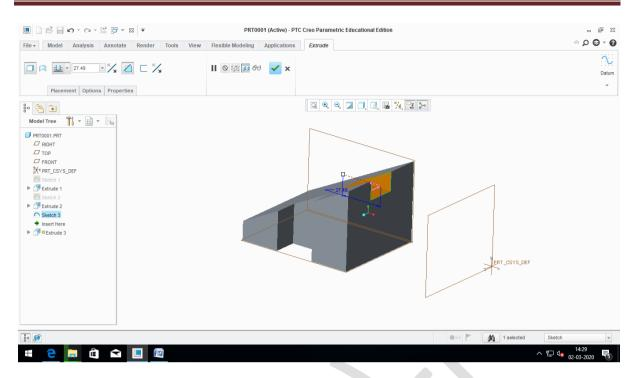
Step8: Extrude the sketch by using Symmetry option and specify the width and direction of extrusion and Click on ok
