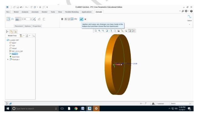
Step7:select the required surface to add the hub and then draw the hub in 2d sketch plane and extrude it by giving the required dimensions
