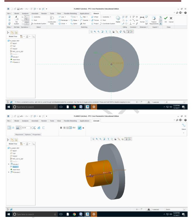
Step 8:select the required surface to add the material and then draw the hub in 2d sketch plane and extrude it by giving the required dimensions
