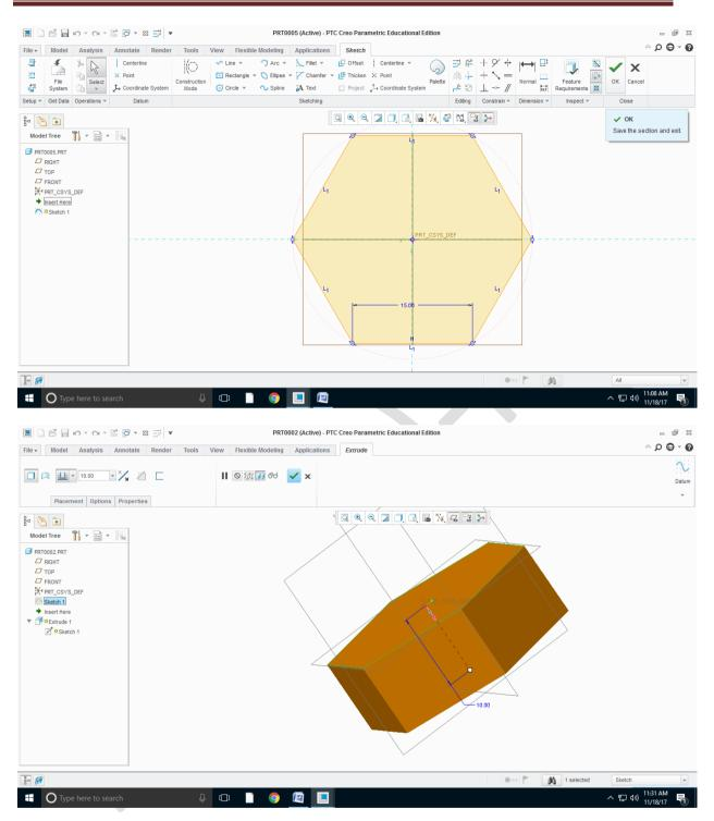
Step13:Select a datum plane as shown in figure and with reference to that draw the required shape to smooth the bolt surface using revolve option nad save it
