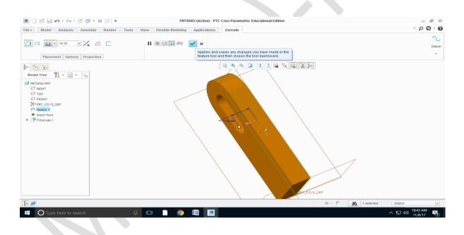
Step7: Select Extrude  $\rightarrow$  Required surface  $\rightarrow$  Sketch View option  $\rightarrow$ Specify references  $\rightarrow$  Draw the required sketch as shown in **Figure.2** Click on ok
