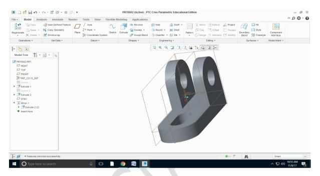
Step10: Round the edges of a part to a specified radius by using Round Command Click on ok
