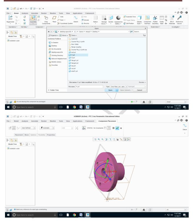
Step 19:Similarly get the  $2^{nd}$  part to do the assembling and select the coinside option and select the parts and axis to be coinsided.
