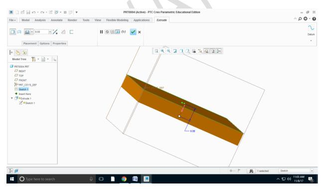
Step7: select the required surface to add the material of the part and also draw the required sketch.
