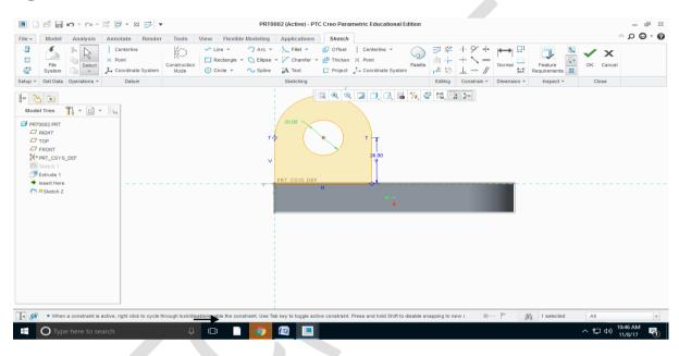
Step8: Extrude the sketch and specify the width and direction of extrusion Click on ok
